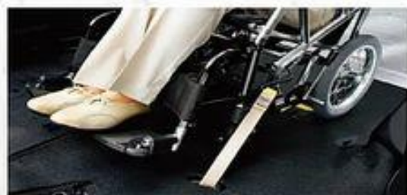
地台防後滑伸縮帶繫輪椅 After-the-Slide Protected Winch
