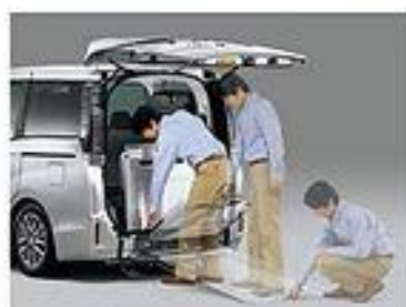
無障礙進出車箱設計式尾板 Easy-Access Designed Rear Platform
